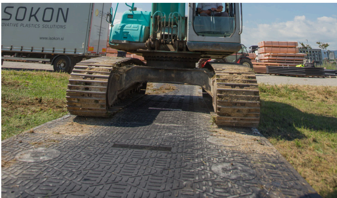
Figure 7a: Caterpielar on Steel side of the mat
