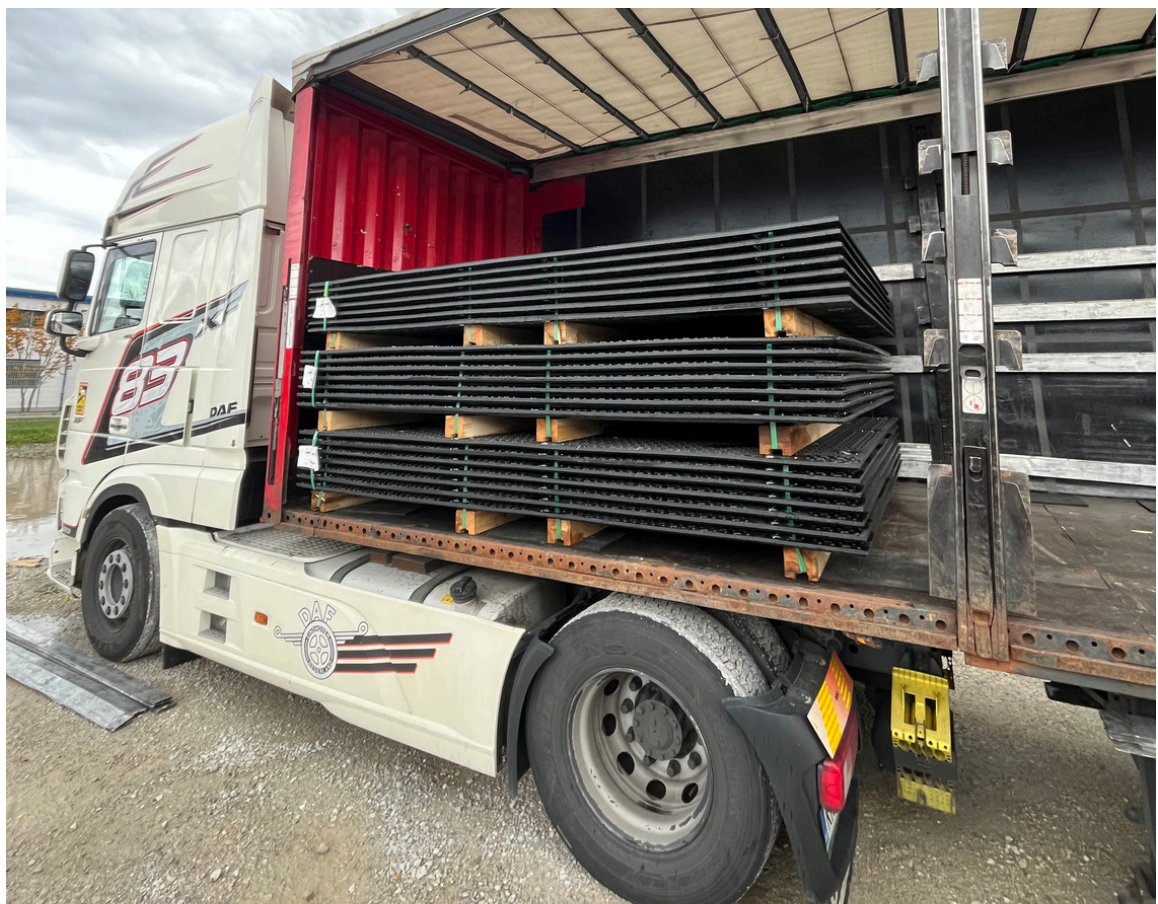
Figure 4j: Proper way of loaded mats on a truck
