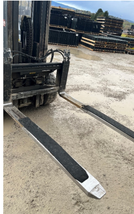
Figure 4c: Extended forks with rubber grips
