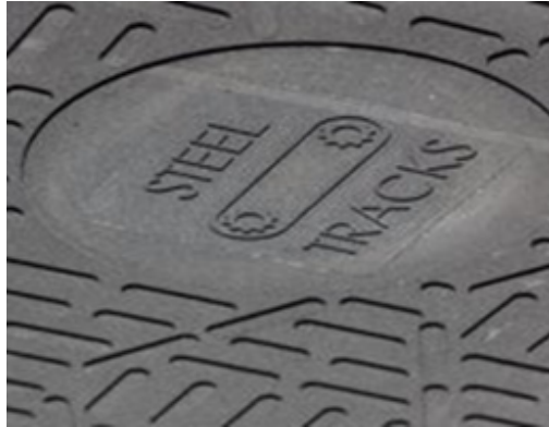
Figure 7b: Steel track symbol
